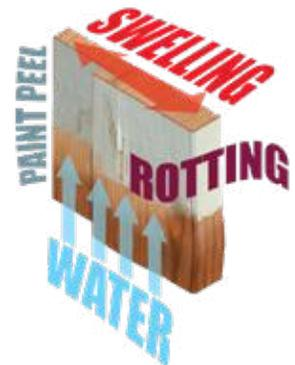
**Shrinking and swelling** occur from changes in relative humidity in the atmosphere. **Water wicks** up through wood fibers resulting in **paint peeling, rot and mold**. Traditional door frames begin to rot within 3-6 months of field installation.
