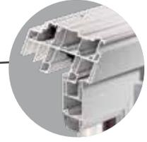
Strong, multi-chamber profiles and 4 7/8" frame depth offer greater thermal efficiency and increased sound abatement. (Endure Patio Door frames have Neopor® insulation).
