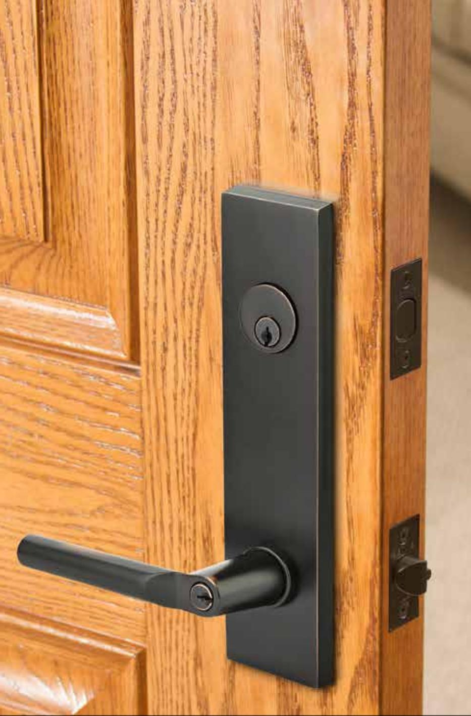
EMTEK's unique Interconnect Device provides the security of a locking deadbolt while providing the means for a panic-proof exit. Turning the interior knob or lever simultaneously retracts both the deadbolt and passage latches.
