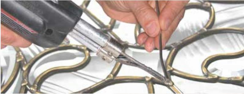
Highly-skilled craftsmen assemble hand-beveled glass accented with a variety of unique glass options by precisely cutting, mitering and soldering each component into artistically designed patterns.
