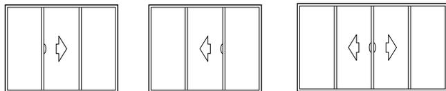
Only available in 2-panel configuration in Certified Wind Load regions. Sidelites and transoms must be installed in a separate opening or use approved engineering mulls.
